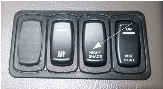
12-Volt Front Drop-Down Night Shade Switch (Located on driver side trim panel) -Typical View
