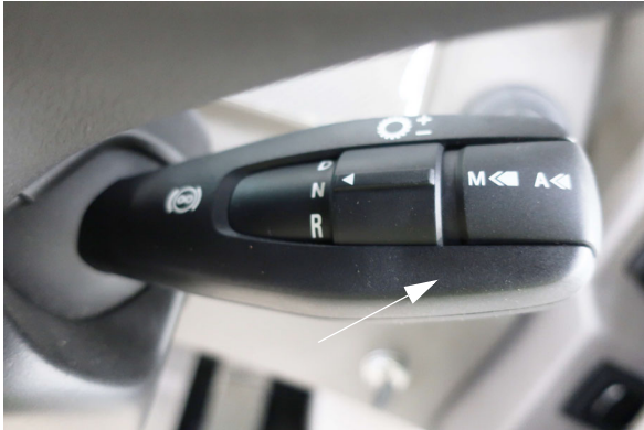
Exhaust Brake Switch (Located on driver's steering column on the right hand stalk switch) -Typical View
