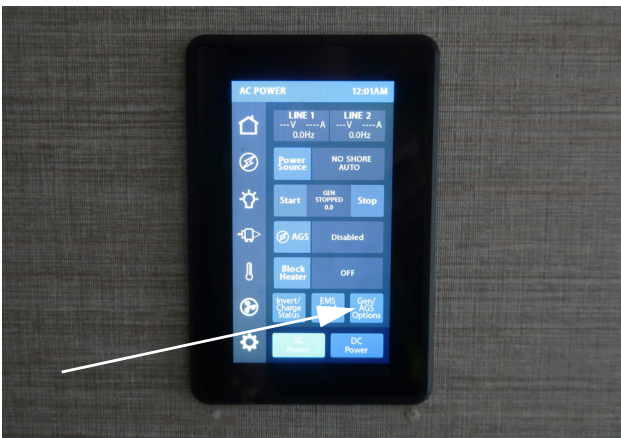
Generator Switch and Hourmeter (Located on multiplex monitor panel “AC” Screen) -Typical View
