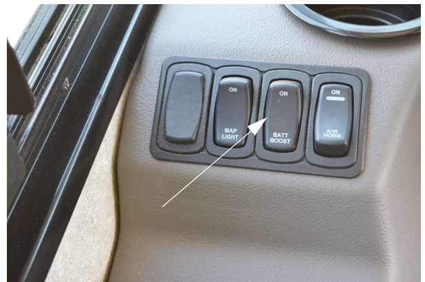
Battery Boost Switch (Located on driver side trim panel) -Typical View
