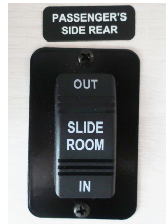
Slideout Switch -Typical View
