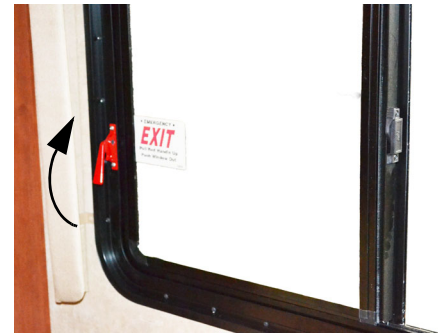
Escape Window (Lift both red safety latch handles UP and push window OUT) *Model 38W -Typical View
